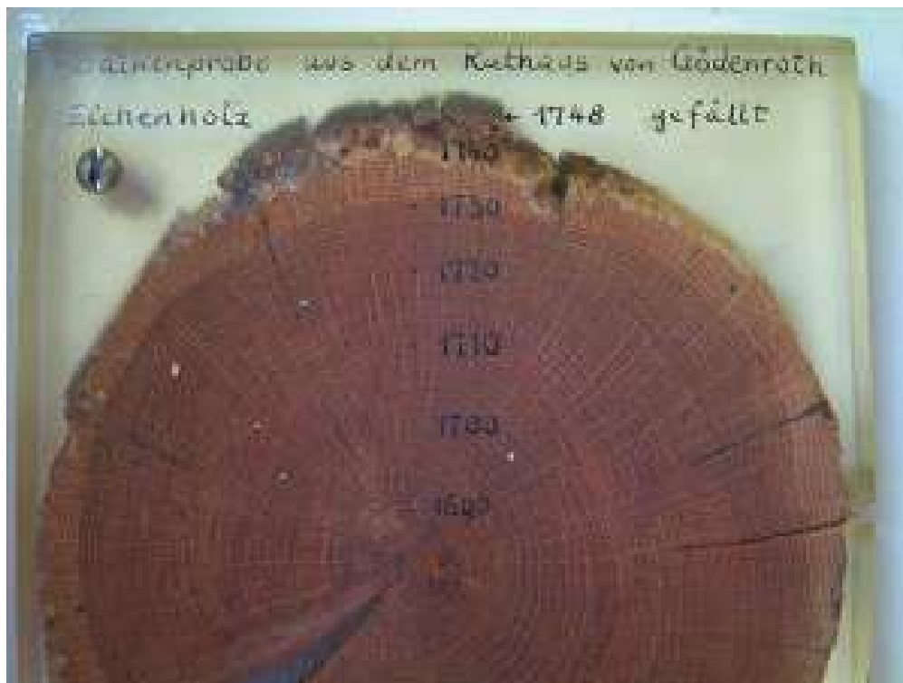
Figure 1.8 Dendrochronology: tree ring dating. “ Dendrochronologie ” by Stefan Kühn is licensed under CC BY-SA 3.0 .
